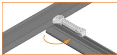
Fig. 4e: CAMO hidden end clamp. Clamp slide into rail channel and the bonding pins contacts the module flange edge.
