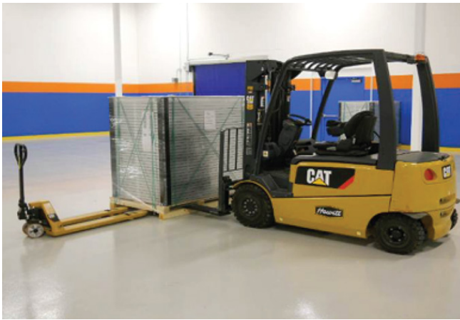
Fig. 10 How to handle the packaging - When using a fork-lift, please ensure the forks go all the way through pallet. The fork length should be a minimum of 1800 mm
